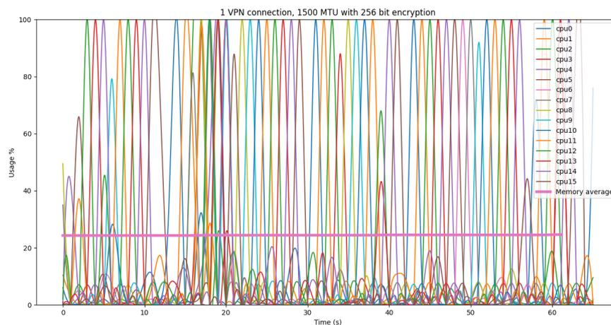
Figure 13: per-core CPU and Memory usage for a 1 VPN 1500 MTU test
