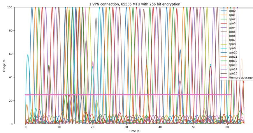
Figure 25: per-core CPU and Memory usage for a 1 VPN 65535 MTU test
