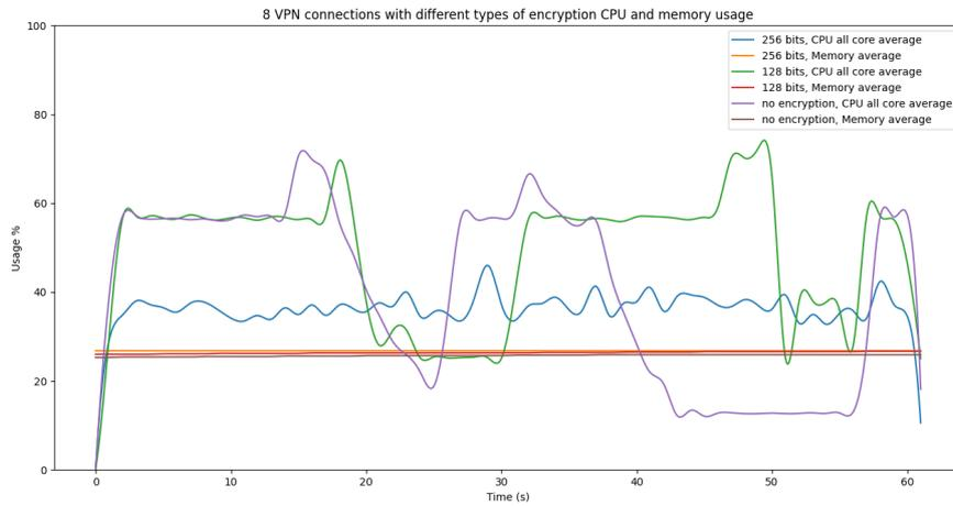
Figure 17: average CPU and Memory usage for an 8 VPN test and multiple ciphers
