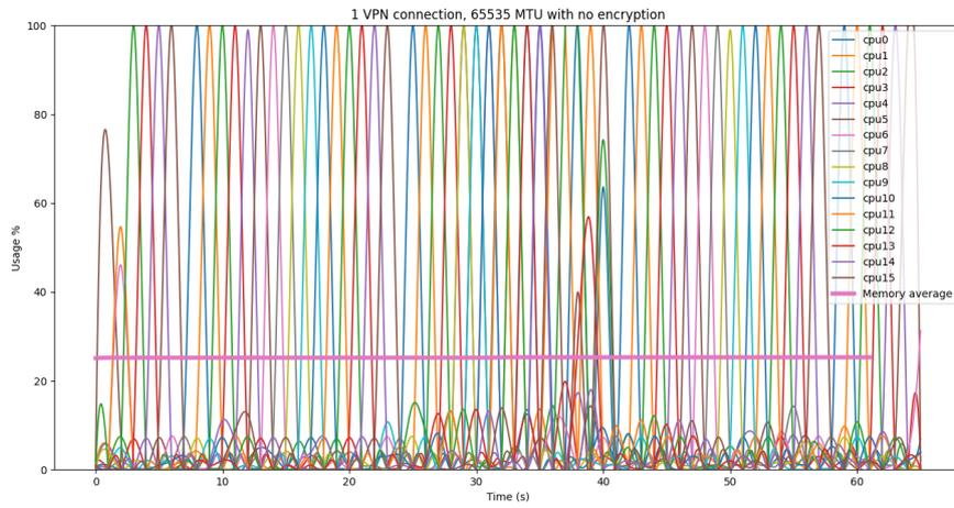
Figure 26: per-core CPU and Memory usage for a 1 VPN 65535 MTU no encryption test
