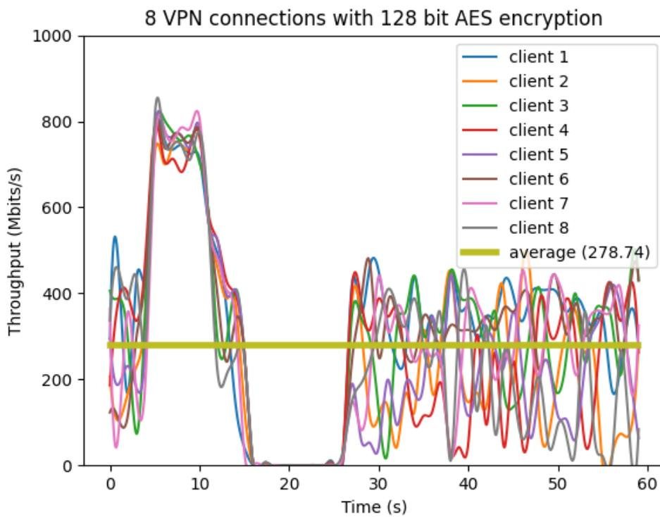
Figure 15: 8 VPN connections with AES-128-CBC encryption
