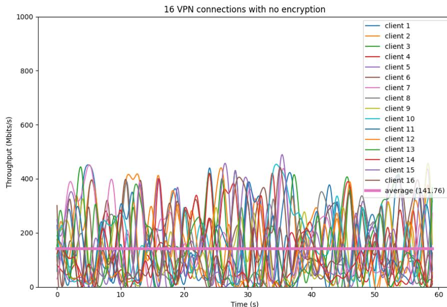
Figure 18: 16 VPN connections with no encryption
