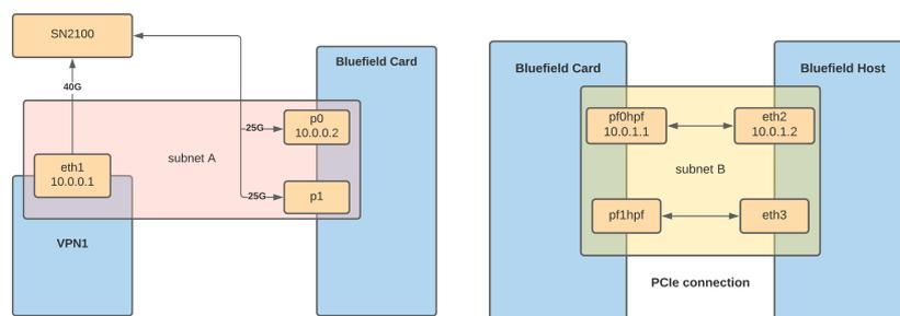
Figure 5: VPN1 machine - Bluefield-1 Card connection through SN2100 switch
