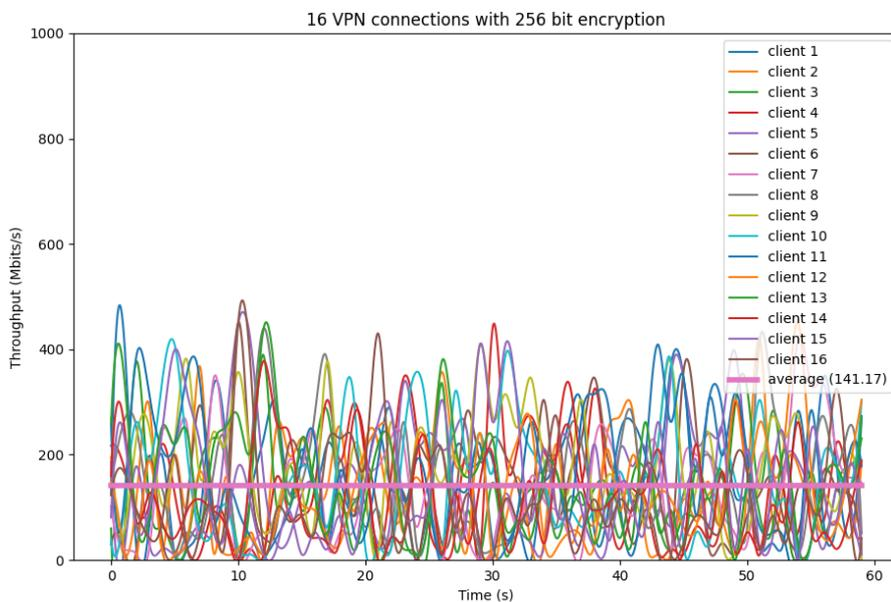
Figure 20: 16 VPN connections with AES-256-CBC encryption
