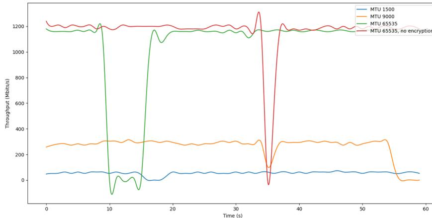
Figure 12: 1 VPN connection from VPN1 to BC with different MTU values
