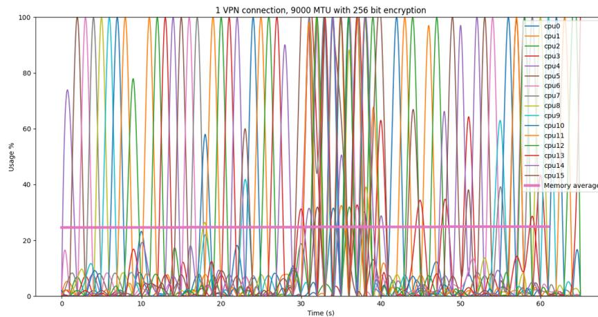
Figure 24: per-core CPU and Memory usage for a 1 VPN 9000 MTU test
