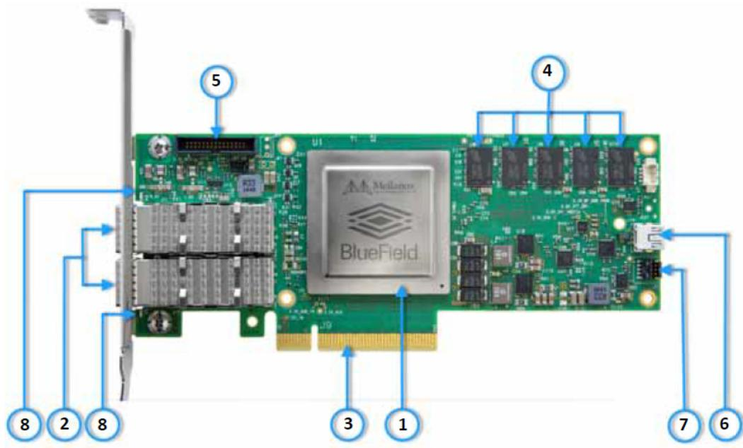
Figure 1: Mellanox Bluefield-1 DPU Layout [1]
