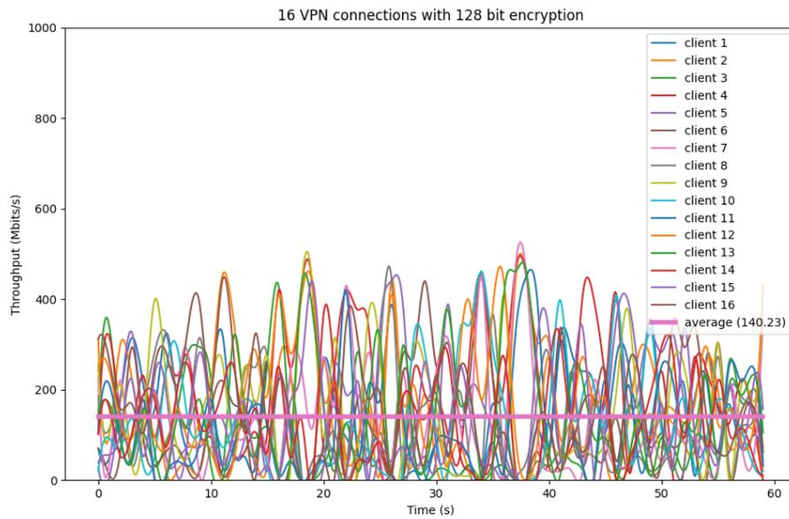
Figure 19: 16 VPN connections with AES-128-CBC encryption
