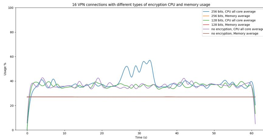
Figure 21: average CPU and Memory usage for a 16 VPN test and multiple ciphers
