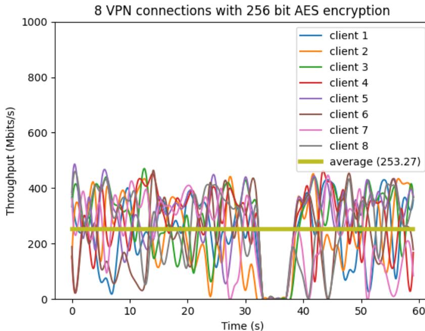
Figure 16: 8 VPN connections with AES-256-CBC encryption
