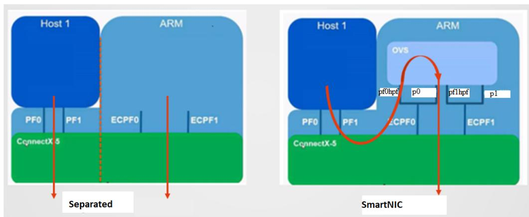
Figure 3: The two modes the DPU can operate in [3]
