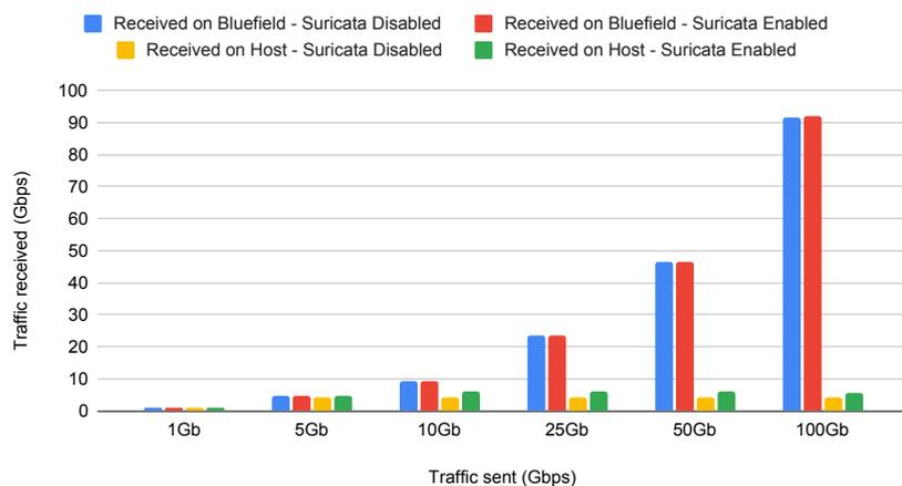
Figure 6: TCP traffic sent and received with a MTU of 1500. When Suricata is running, it runs in IDS mode alongside Ovs and is only alerting.
