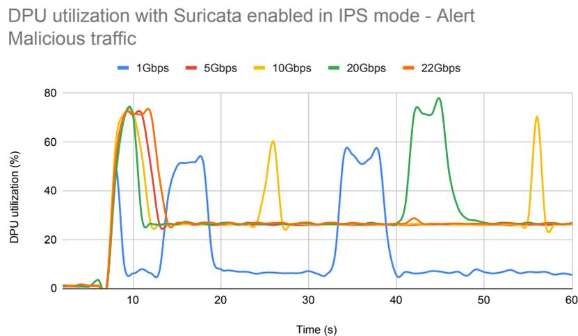
Figure 17: DPU utilization when Suricata enabled in IPS mode, only alerting. Sending malicious traffic.
