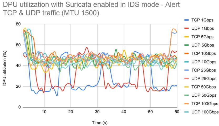
Figure 9: DPU utilization when Suricata is enabled in IDS mode running alongside OvS. Sending TCP & UDP traffic with a MTU of 1500.
