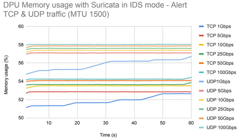
Figure 11: Memory usage when Suricata is enabled in IDS mode running alongside OvS. Sending TCP & UDP traffic with a MTU of 1500.
