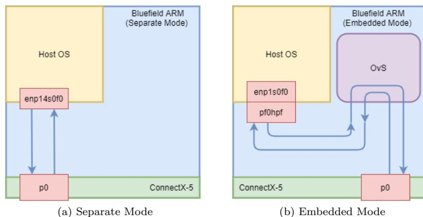
Figure 1: The two modes of operation on the BlueField
