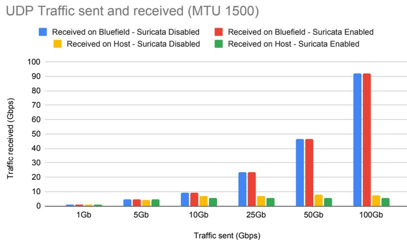
Figure 4: UDP traffic sent and received with a MTU of 1500. When Suricata is running, it runs in IDS mode alongside Ovs and is only alerting.
