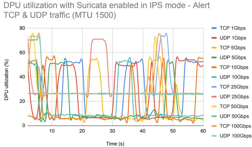
Figure 14: DPU utilization when Suricata enabled in IPS mode, only alerting. Sending TCP & UDP traffic with a MTU of 1500.
