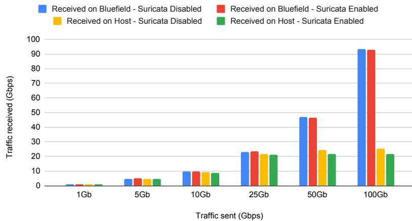
Figure 5: UDP traffic sent and received with a MTU of 9000. When Suricata is running, it runs in IDS mode alongside Ovs and is only alerting.
