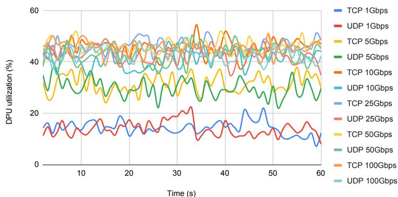
Figure 8: DPU utilization when Suricata is disabled and OvS enabled. Sending TCP & UDP traffic with a MTU of 1500.
