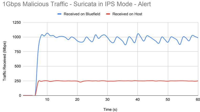
Figure 16: Malicious traffic received on the BlueField and host. Suricata is running in IPS mode and is only alerting.
