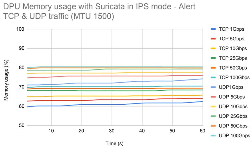
Figure 15: Memory usage when Suricata enabled in IPS mode, only alerting. Sending TCP & UDP traffic with a MTU of 1500.
