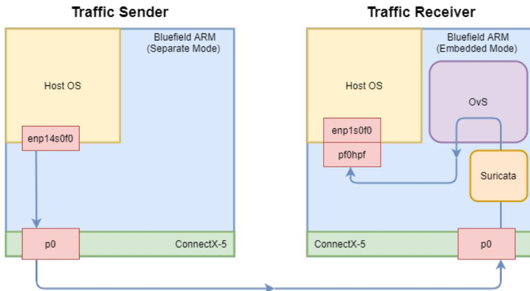
Figure 3: Overview of the experimental setup with Suricata installed on the receiving DPU in embedded mode
