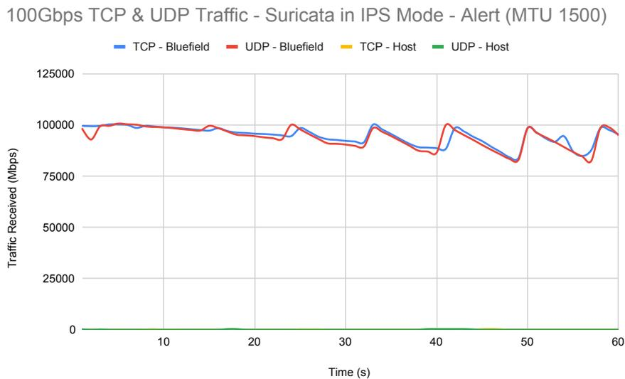
Figure 13: TCP and UDP traffic with a MTU of 1500 received on the BlueField and host. Suricata is running in IPS mode and is only alerting.
