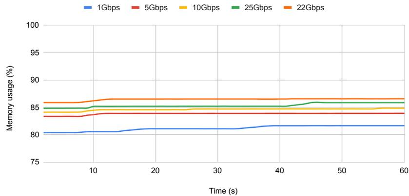
Figure 18: Memory usage when Suricata enabled in IPS mode, only alerting. Sending malicious traffic.
