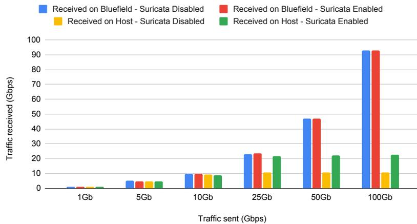
Figure 7: TCP traffic sent and received with a MTU of 9000. When Suricata is running, it runs in IDS mode alongside OvS and is only alerting.
