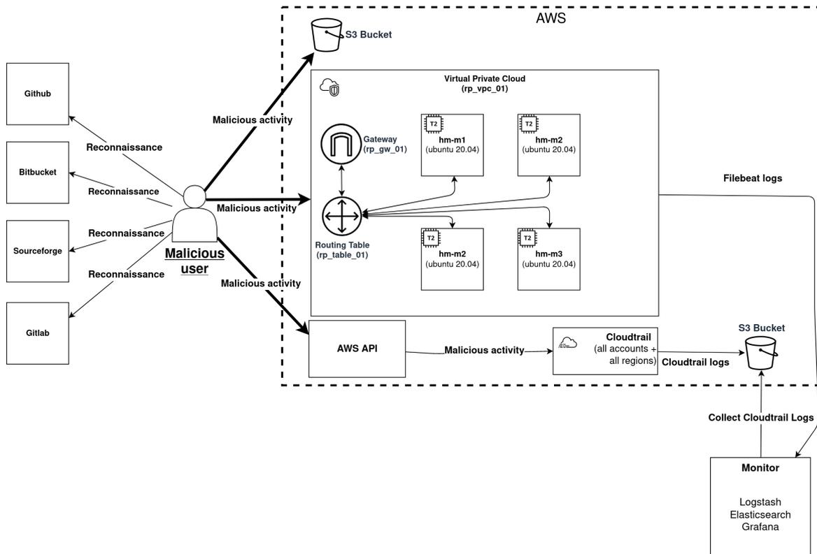
Figure 2: Overview of the AWS experimental environment.
