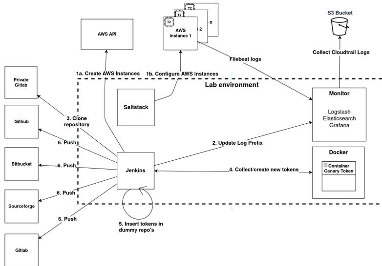
Figure 1: Overview of the Lab environment setup for the experiments detailing the steps a Jenkins pipeline takes to setup an experiment.
