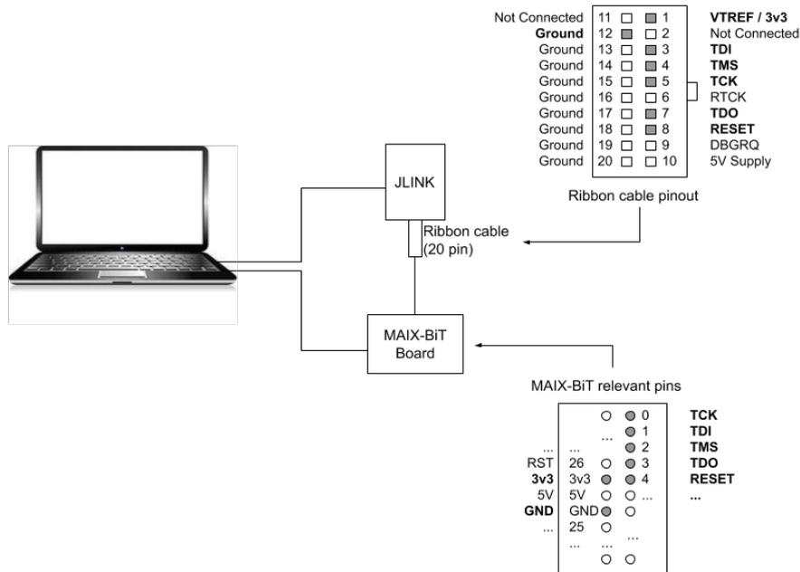
Figure 1: The debugging setup, including the pinout. The pins that need to be connected are listed in bold.
