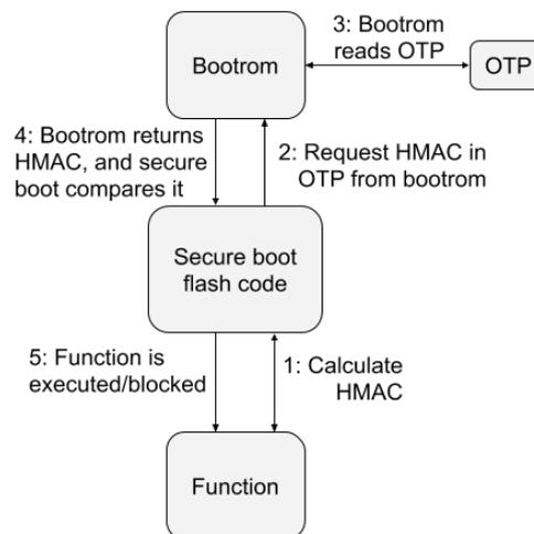
Figure 2: The proposed secure boot implementation on the Kendryte K210.
