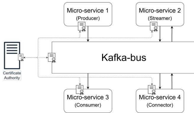
Figure 2: Basic Kafka environment with certificate-based encryption and authentication.
