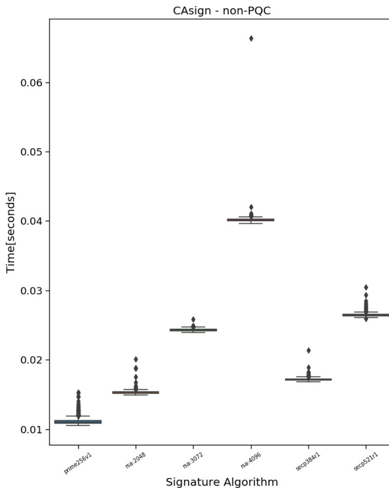
Figure 8: Time measurements for generating signing using classical cryptography algorithms.
