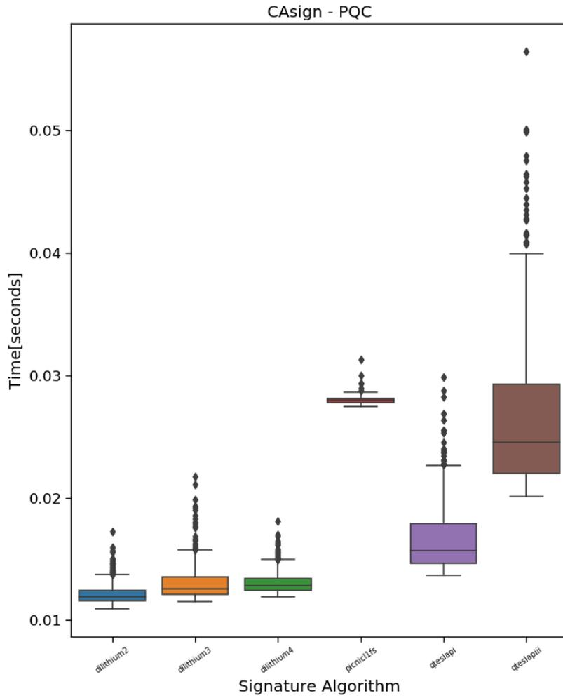
Figure 11: Time measurements for generating signing PQC algorithms.
