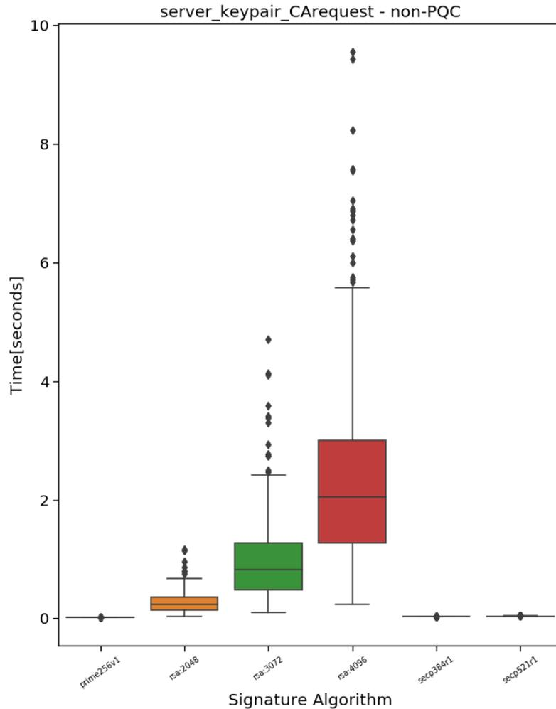
Figure 7: Generating certificates with classical cryptography
