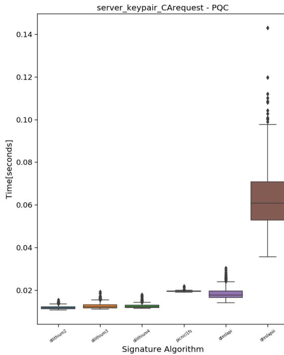
Figure 10: Time measurements for generating certificates using PQC algorithms.
