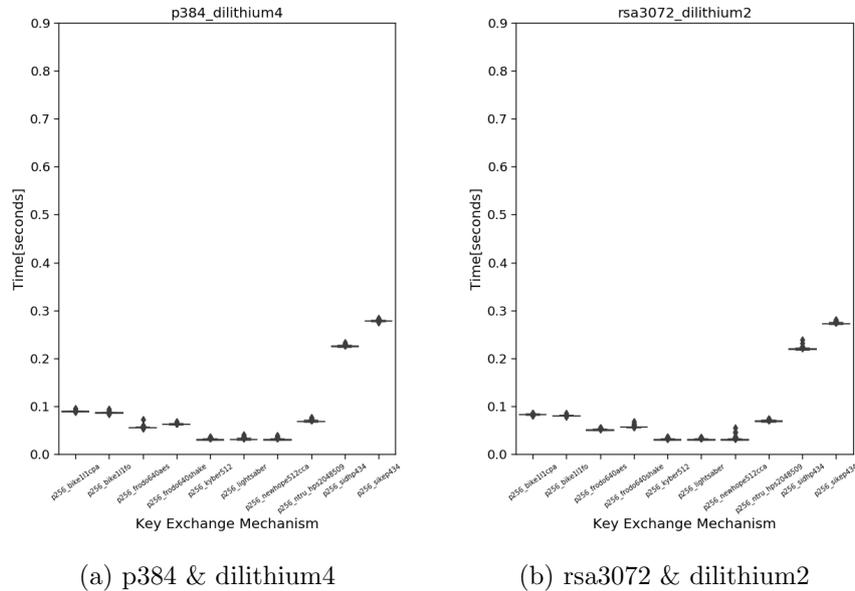
Figure 6: Measured handshake times for hybrid post quantum cryptography
