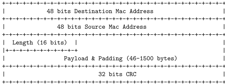
Figure 8: Ethernet Packet Header [9]
