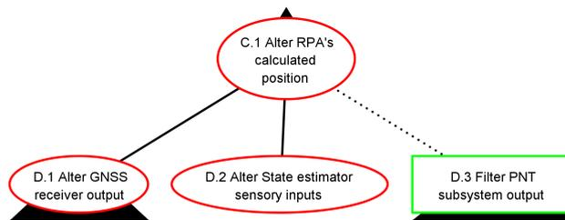
Figure 6.2: Sensor based attacks. As indicated by the black triangle on the top node (C.1), parent nodes are hidden. This sub-tree connects to node B.2.
