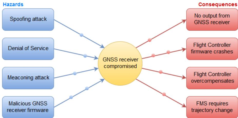
Figure 9.1: Compromised GNSS receiver scenarios. In the Bowtie model, *Hazards* mentioned on the left lead to a *feared event* located at the centre. The feared event in turn leads to possible *Consequences* shown on the right. Blue and red spheres represent *preventative* and *reactive* controls respectively.
