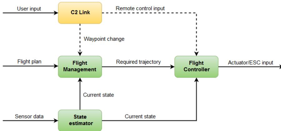
Figure 5.2: Core processing components aboard the RPA (shown in green) and shared components between RPA and RPS (shown in yellow).
