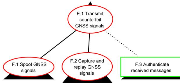
Figure 6.4: Counterfeit signal based attacks. This sub-tree connects to node D.1.
