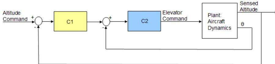
Figure 5.1: Elevator feedback loop [Mat]
