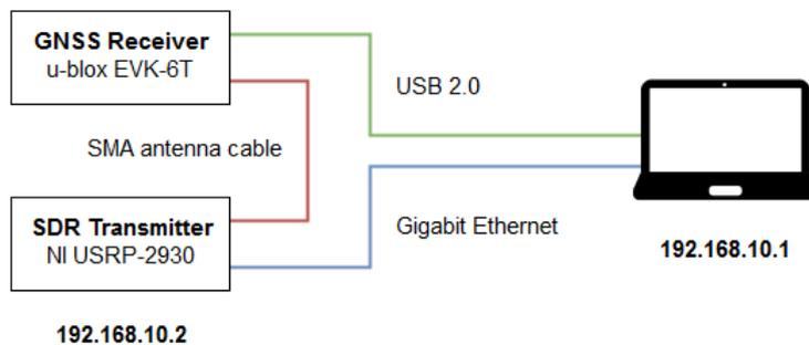
Figure 4.1: Experiment set-up
