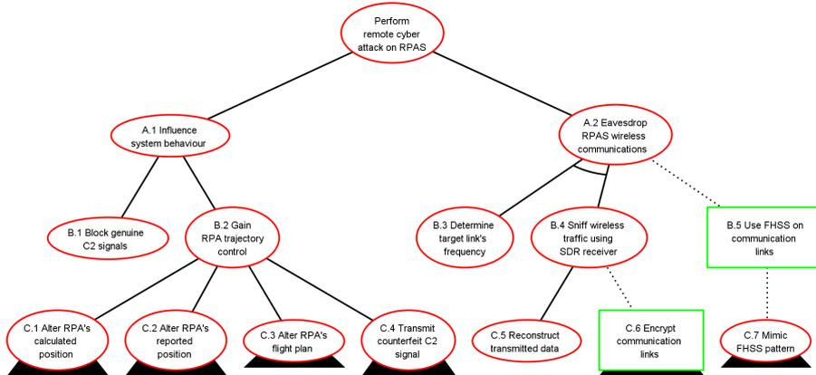
Figure 6.1: Sub-tree showing wireless threats. Connecting (arc) lines between refinements depict conjunction (i.e. all sub-goals must be achieved). The presence of a black triangular shape beneath the node indicates the existence of further child nodes.
