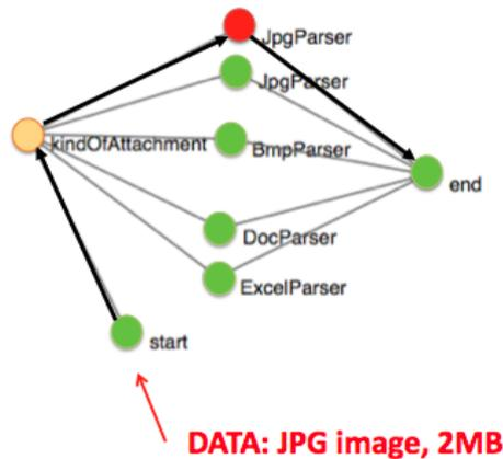
Figure 7: A JPG data item generates a certain load on the nodes of the functions it hits.
