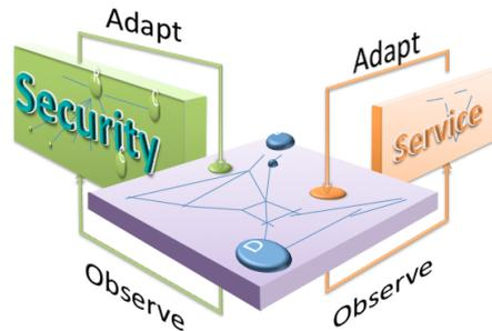
Figure 3: A security control loop and a service control loop observe and adapt the network [Image: Robert Meijer].
