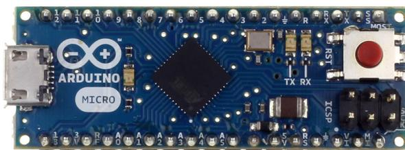
Figure 1: Arduino Micro Front; source [3]
