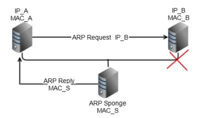
Figure 1.3: ARP sponge behaviour in the case of a down node
