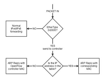
Figure 3.2: ARP processing flowchart
