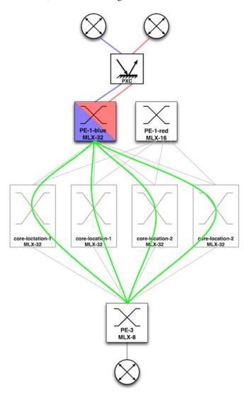
Figure 1.2: Failover in case of PE failure
