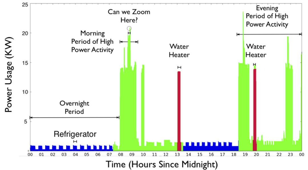
Basic patterns can be inferred with minimal analysis, even with power measurements every 30 seconds.
